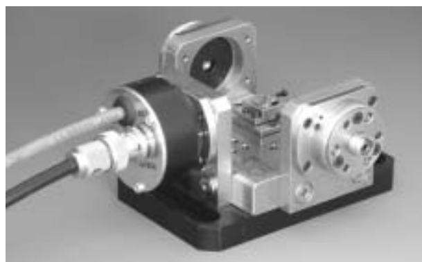
Tap Beamsplitter and DetectorPort on typical FiberBench
