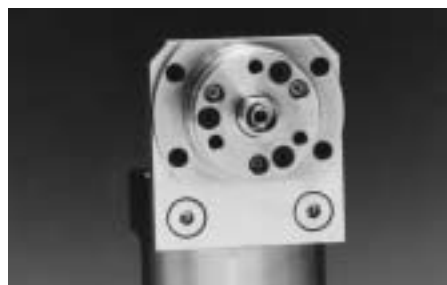
FiberPort with cover removed, face view, showing coupling adjust-and-lock screws
