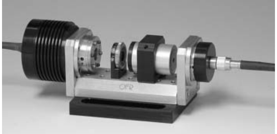
IO-P-FTB-9-980-X, Laser-to-Fiber Isolator. Note that alignment of plane of polarization is achieved with a 1/2-wave retarder (RZB-1/2-980, page FO-15) mounted in RCB Rotation Base (page FO-11).
