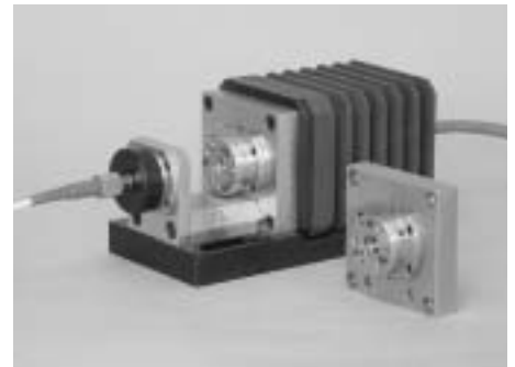
PAL-TO3-830 mounted on customer's heatsink.
