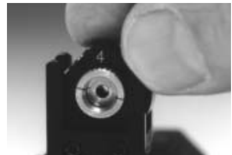
SOP Module is manually set in 4 positions.
